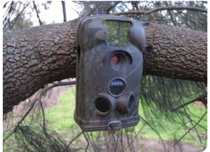
In this case, pedestrians were counted for two weeks. Camera batteries can last for approximately 5,000 frames, so the period of recording depends on the approximate number of pedestrians. Batteries can be replaced if longer time recording is required.
